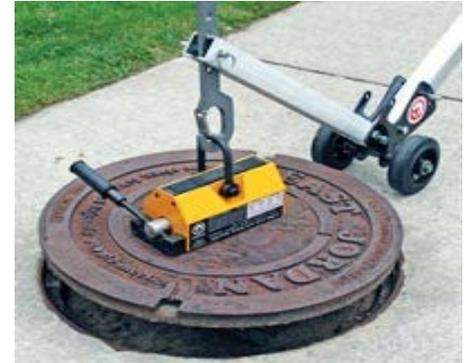
Set up the site with the necessary cones or other traffic warning methods including, if needed, a flagger. When in a work zone ensure that all workers are wearing the proper safety vest, good gloves and safety boots. Set up the lifter’s position so that the wind is at the lifter’s back, blowing dust and sewer gasses away from them.
