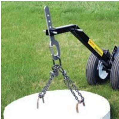
Clean off the top of the manhole cover, as it may be covered with a layer of dirt, debris and other material. You can use a heavy-duty broom if the debris is loose, or you may need a shovel if the debris has become compacted. Tap the cover with a maul to loosen it. If the cover is solid, you should monitor for flammable gasses around the edges or in pick holes before opening.
