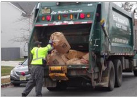
Leaf collection is a Mobile Work Zone. Establish traffic control according to the MUTCD. At a minimum, high intensity amber warning lights must be visible to motorists approaching from either direction.
